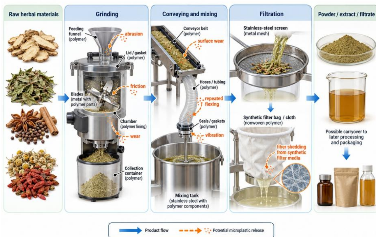
Figure 3. Schematic diagram of secondary microplastic contamination during grinding, conveying, mixing, and filtration.
