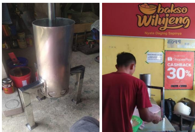
Gambar 3. Alat pencetak bakso ( meatballs maker )
